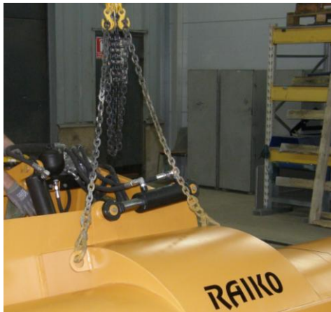
Picture 1. Lifting with lugs
