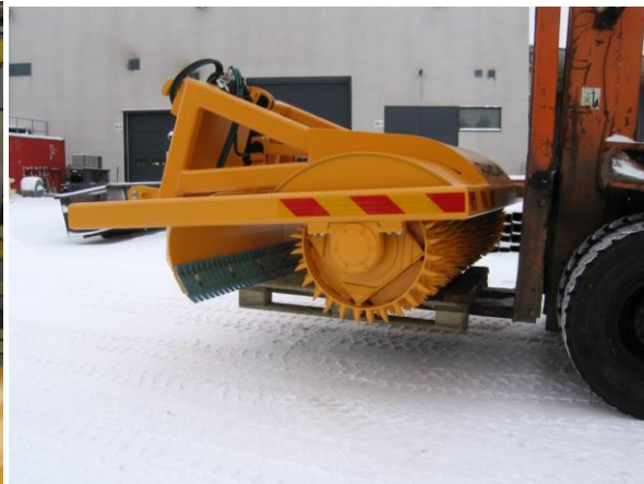
Picture 2. Lifting with a forklift
