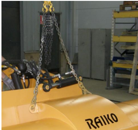
Picture 1. Lifting with lugs
