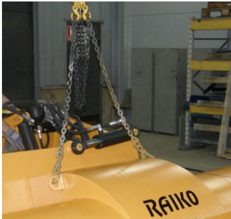
Picture 1. Lifting with lugs
