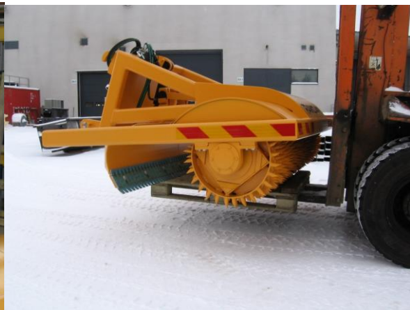
Picture 2. Lifting with a forklift
