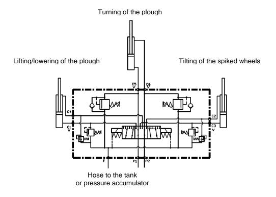
Picture 1. Connection diagram of the hydraulics unit.
